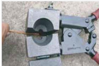
4 Fit conductors and ground rod snugly into the mould and lock the handle clamp Always make sure the mould is in a level position
